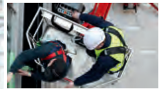
200kg basket capacity in the entire working area - sufficient for 2 persons including tools and material.
