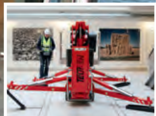
Simple, safe and quick - Fully automatic self-levelling at the push of a button
