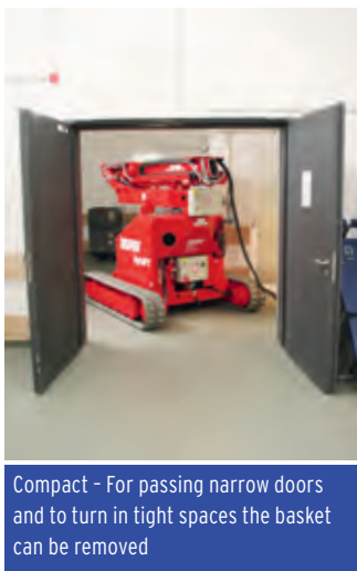
With a width of 1,78m and a total weight of 2985kg the LE012T fits into standard freight elevators.
