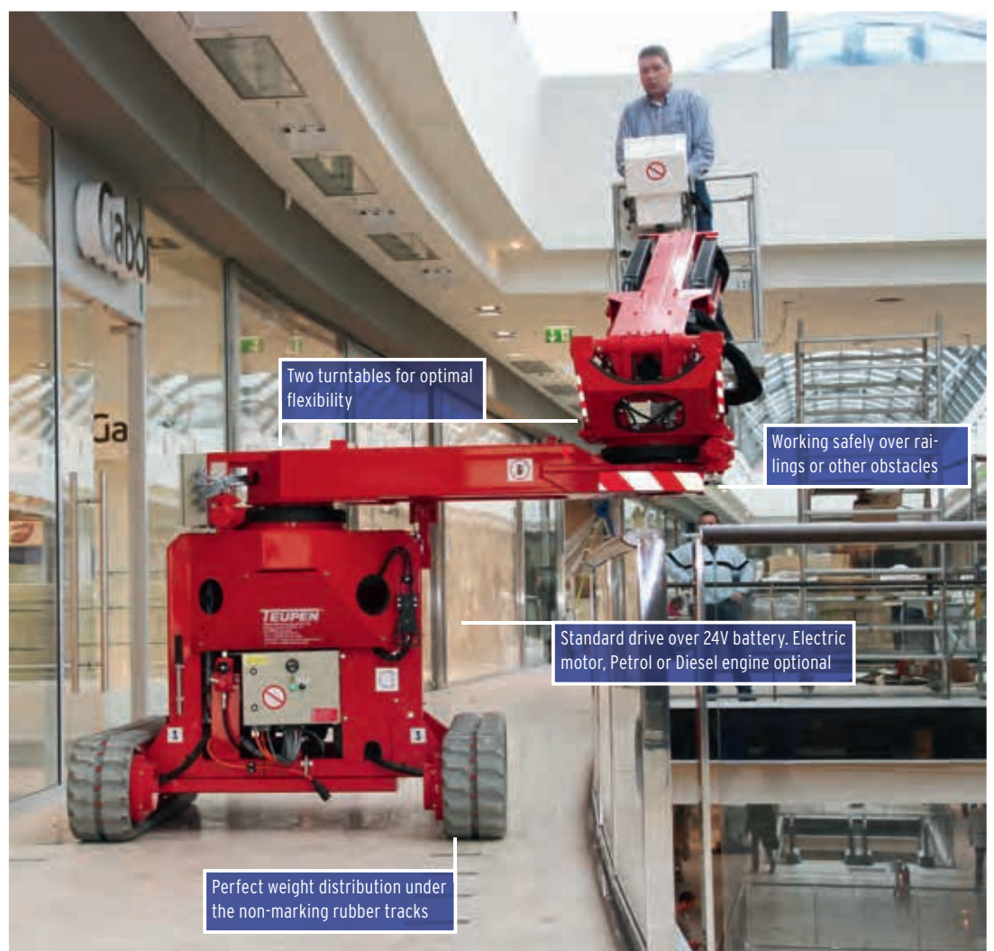
With a width of 1,78m and a total weight of 2985kg the LE012T fits into standard freight elevators.
